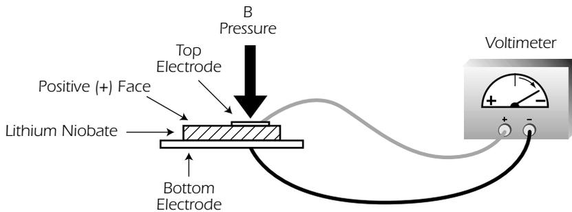
**FIGURE 2. CRYSTAL POLARITY MEASUREMENT**
