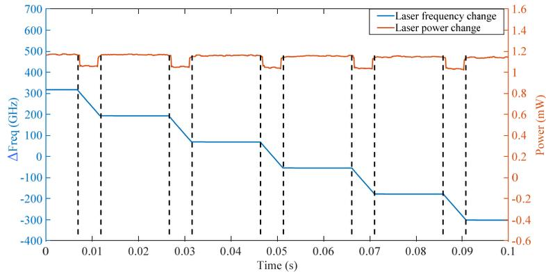
**Figure 4 Step-modulated laser ( $v=10\text{nm/s}$  ,  $d\lambda=1\text{nm}$ )**
