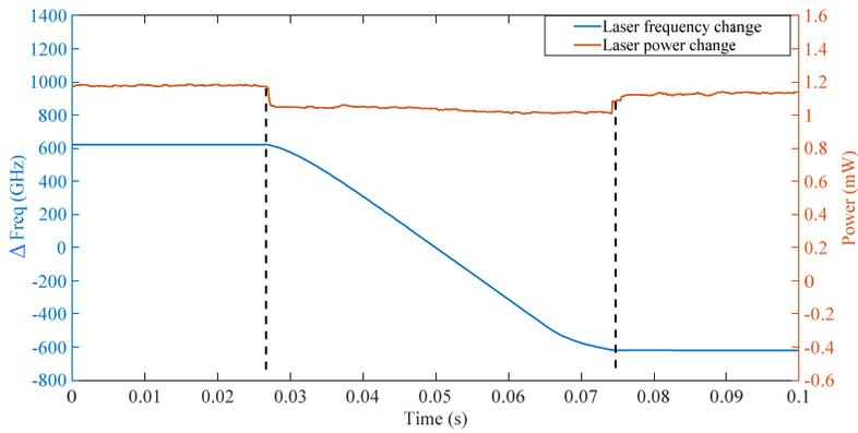
**Figure 5 Continuously modulated laser ( $v=50\text{nm/s}$  ,  $d\lambda=10\text{nm}$ )**
