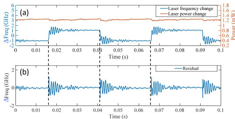
**Figure 3 Square wave laser frequency modulation**
