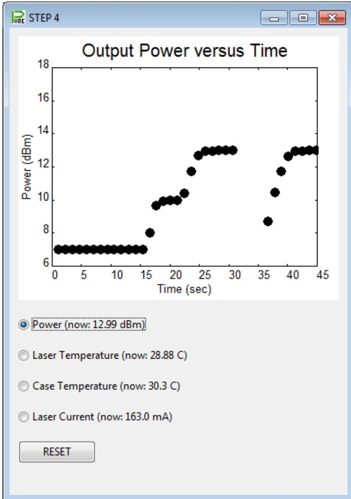
Figure 9: Step 4 window – graphs (shows laser set at 7dBm, power increased to 10 and 13dBm and then switched to different frequency)
