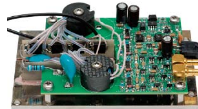
Fig. 11. OEM version of DPS/DPD series driver with conductive pad. Suitable for repetition rate up to 50 kHz
