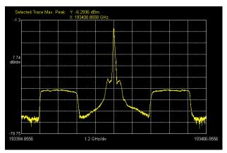
In the example below, **8** OFDM channels are shown. Aligning these signals to avoid overlapping with a normal OSA requires constantly switching off channels to see the carrier wavelength and taking leaps of faith on the unseen spectrum, whereas with BOSA all the information is seen in a single scan.
