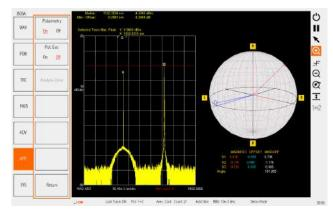
The continuous evolution of the state of polarization can also be measured. Select a portion of the measured span to plot the evolution of the SOP with high resolution.
