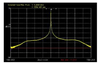
In this measurement the spectral shape of a DFB laser is shown. Just by measuring the spectral linewidth at different bias currents the linewidth enhancement factor can be extracted.
