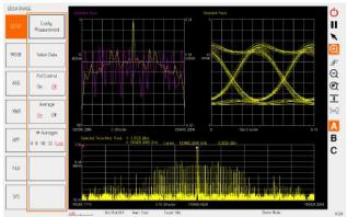
BOSA option 440 (BOSAphase) turns the BOSA into an **Optical Complex Spectrum Analyzer** (OCSA) which is another patented technology by Aragon Photonics.
